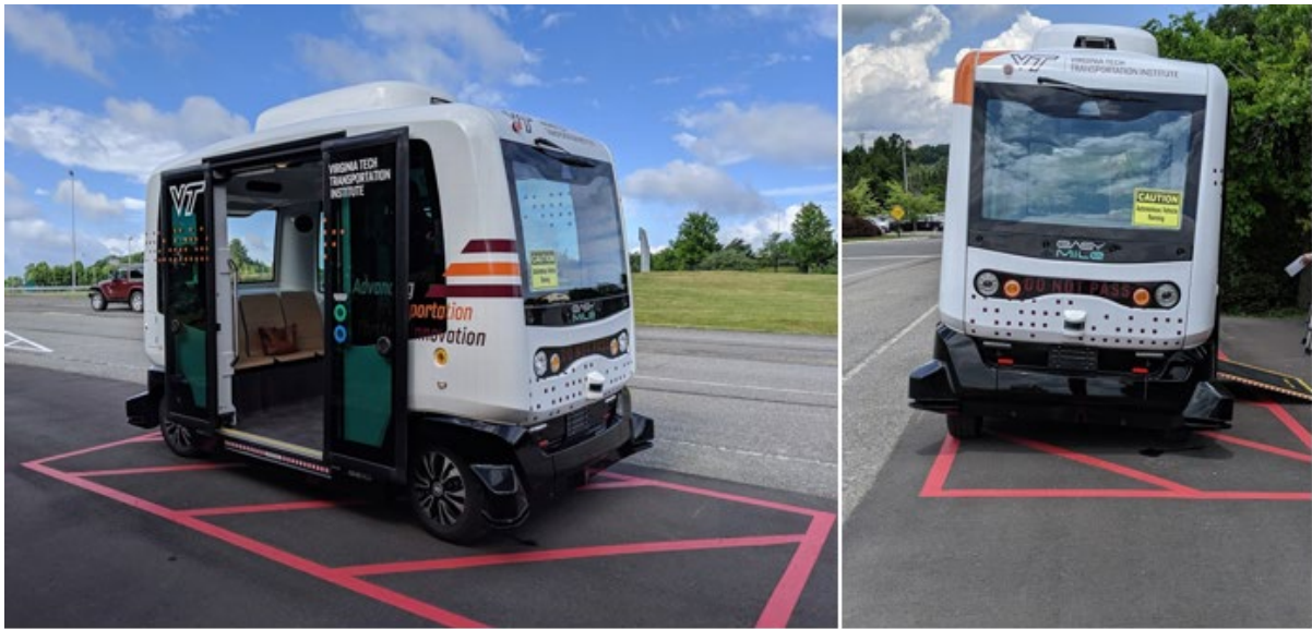
Figure 3. Views of VTTI’s EasyMile LSAV parked with doors open (left) and in leaning mode with entry ramp deployed (right).
