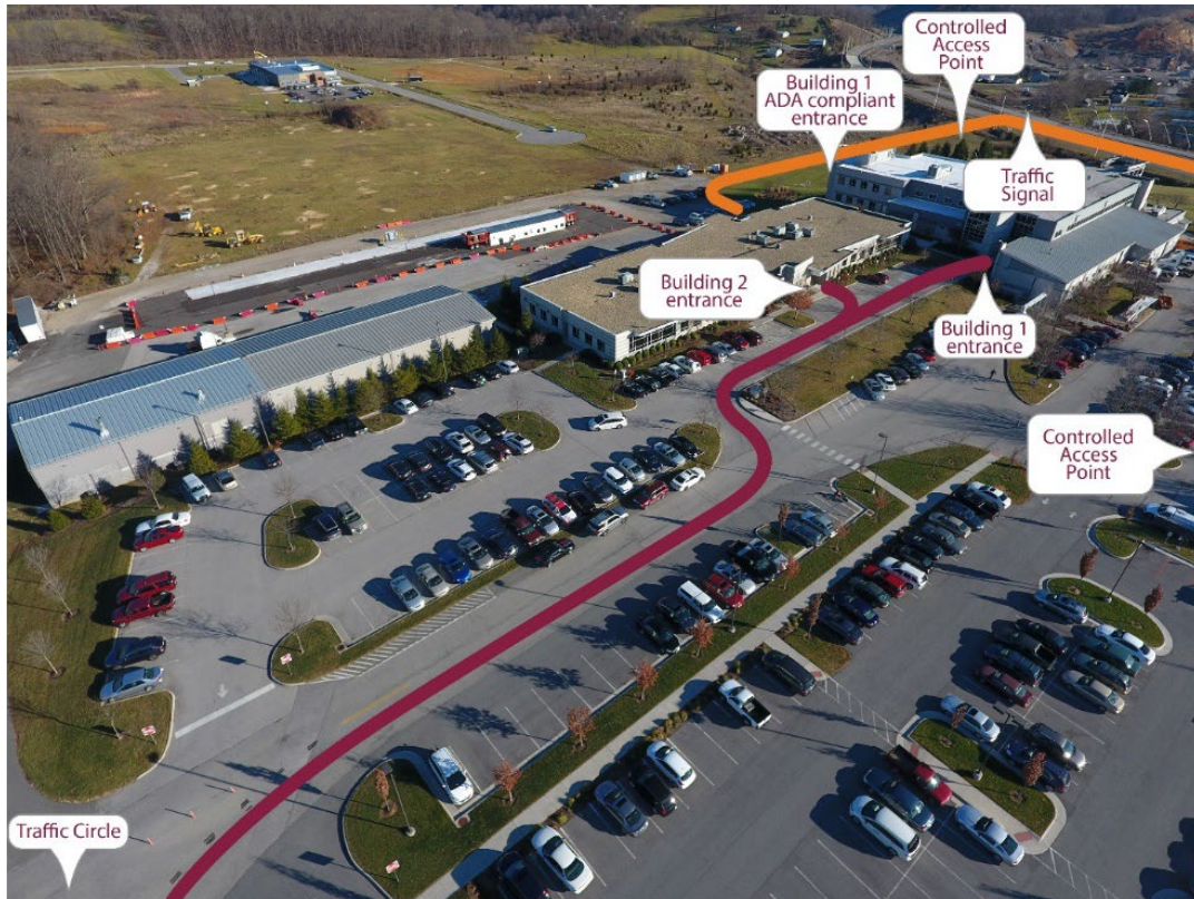
Figure 6. An aerial view of the LSAV’s route through VTTI’s parking area with termination at the front entry of the main building lobby (maroon line).
