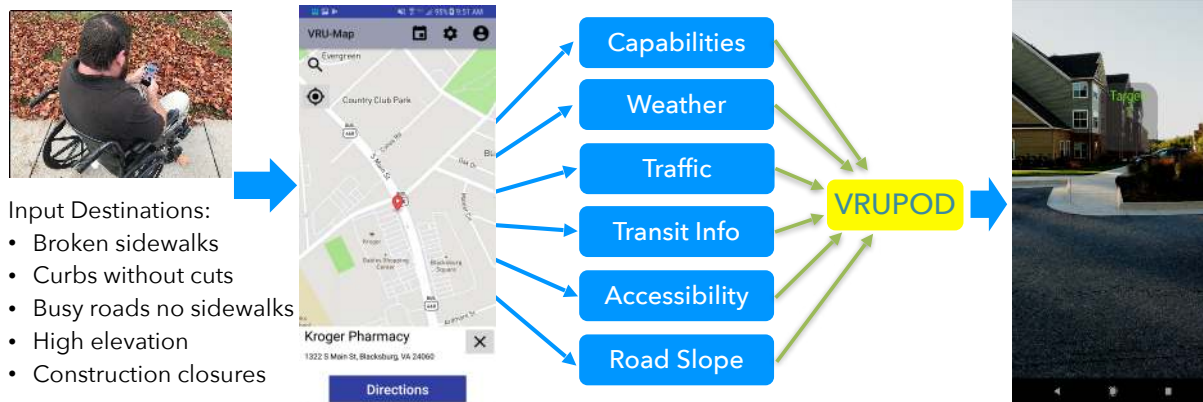
Figure 1: Vulnerable Road User Mobility Assistance Platform (VRUMAP) and the Role of VRUPOD
